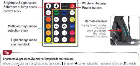
When single color light or whole white light is on, ↑ brighter/↓ darker; when the multicolor light is on, ↑ the ligh runs faster/↓ the light runs slower. When you press "IC Set" button, you can choose how many lamp beads wor Press "IC Set" button again to end the setting.
