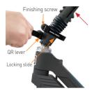
**1. Raise the handle post(Steering tube)** Release the QR lever, raise the locking slide upwards, raise the handle post, then lower the locking slide downward.
